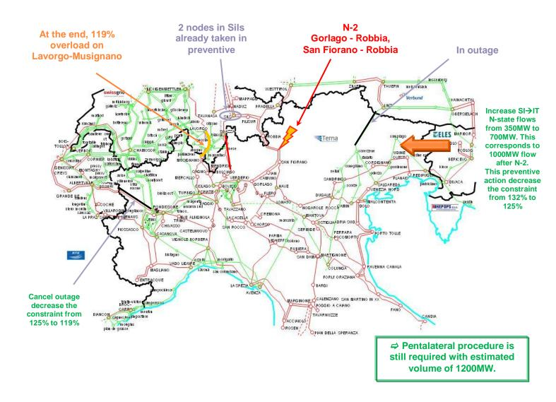
Thanks to those actions (2 nodes in Sils, flows increase on SI border, cancel outage on Albertvile – Rondisonne 1) and to a big pentalateral reduction, the situation was manageable in real time avoiding cascading effect in case of N-2 from Switzerland.
