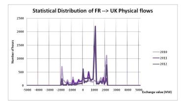
The curves show a long period exchanges around 1000MW. This is due to maintenance on IFA cables, which force us to stay with only one bipole (Maximum 1000MW per bipole).
