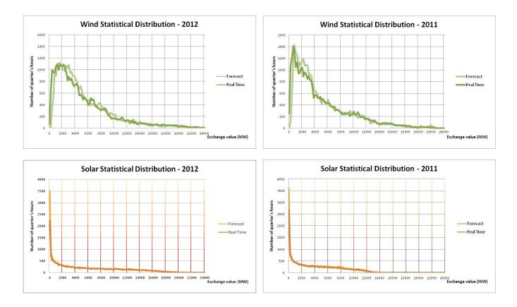
Wind infeed was a little bit higher than in 2011, with more times spent up than 4000MW of generation.
