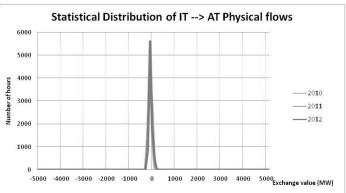
In 2012, with the PST regulation, loopflows were within the normal range [-1200 MW; +1000 MW] 95.5% of the time (93% in 2011).
